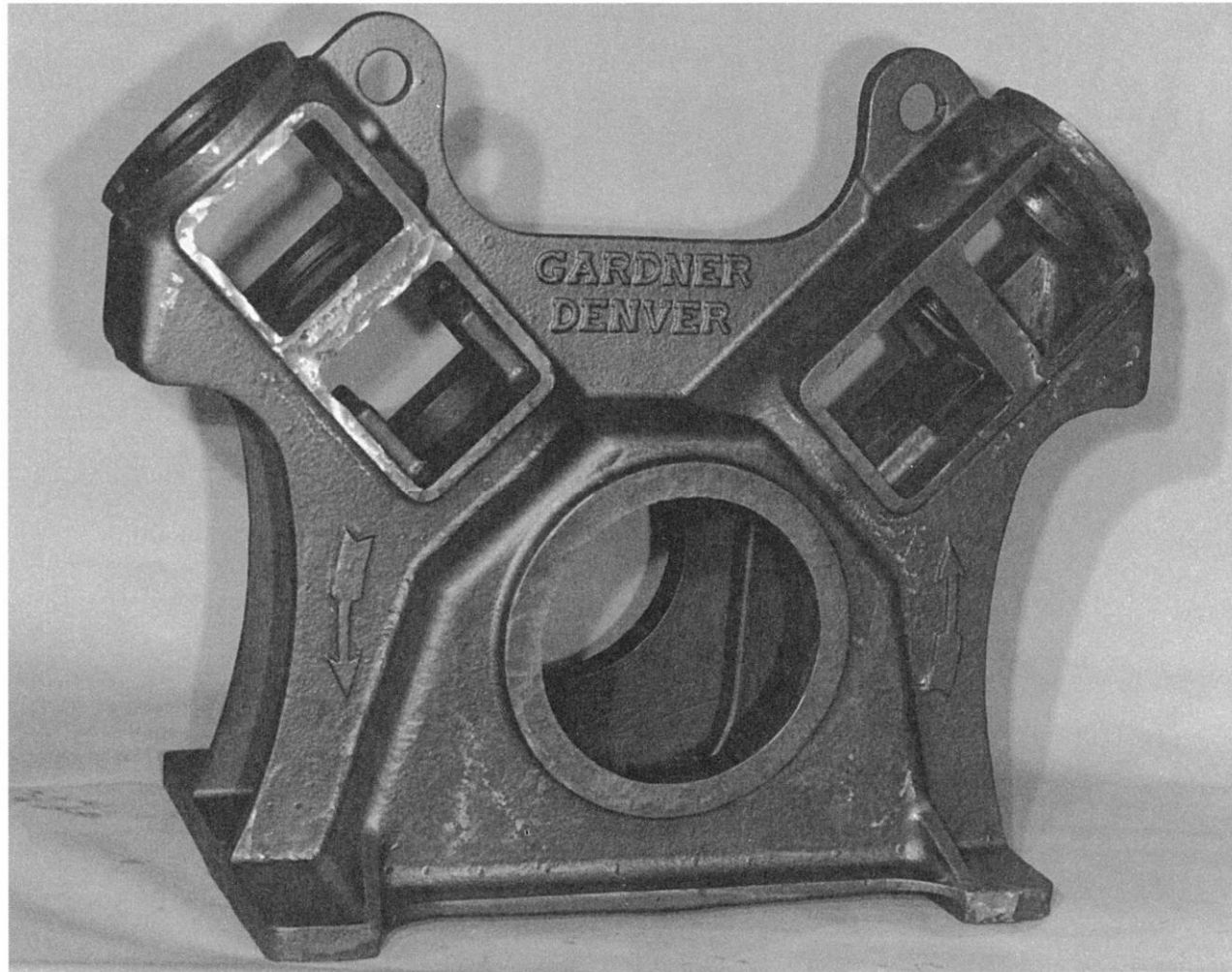
A large sand casting weighing over 680 kg (1500 lb) for an air compressor frame
