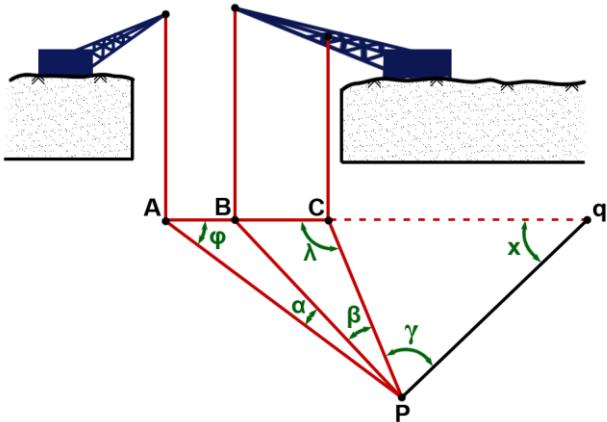
$$\begin{array}{l|l} A & \left| \begin{array}{l} 100 \\ 100 \end{array} \right. \\ \hline & , \\ \alpha & 31^{\circ}30'12'' \end{array}, \quad \begin{array}{l|l} B & \left| \begin{array}{l} 105.32 \\ 104.55 \end{array} \right. \\ \hline & , \\ \beta & 42^{\circ}51'13'' \end{array}, \quad \begin{array}{l|l} C & \left| \begin{array}{l} 110.87 \\ 109.29 \end{array} \right. \\ \hline & , \\ \gamma & 50^{\circ}18'08'' \end{array}$$
