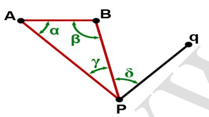
$$\begin{aligned} \overline{AB} &= (\overline{PA}^2 + \overline{PB}^2 - 2 \times \overline{PA} \times \overline{PB} \cos \gamma)^{0.5} \\ \frac{\sin \alpha}{PB} &= \frac{\sin \gamma}{AB} \Rightarrow \alpha = \sin^{-1} \left( \frac{PB \times \sin \gamma}{AB} \right) \\ \frac{\sin \beta}{PA} &= \frac{\sin \gamma}{AB} \Rightarrow \beta = \sin^{-1} \left( \frac{PA \times \sin \gamma}{AB} \right) \end{aligned}$$
