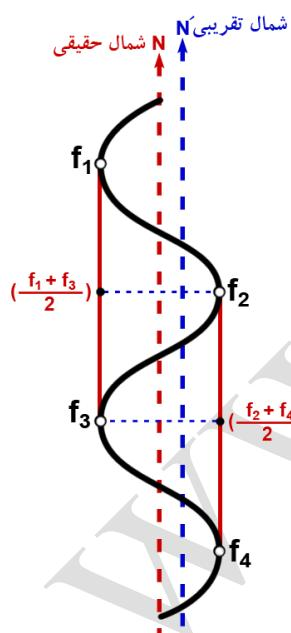
$$\begin{aligned} N_1 &= \frac{1}{2} \left( \frac{f_1 + f_3}{2} + f_2 \right) \\ N_2 &= \frac{1}{2} \left( \frac{f_2 + f_4}{2} + f_3 \right) \\ &\vdots \quad \vdots \quad \vdots \end{aligned} \Rightarrow N = \frac{1}{N} \sum_{i=1}^n N_i$$
