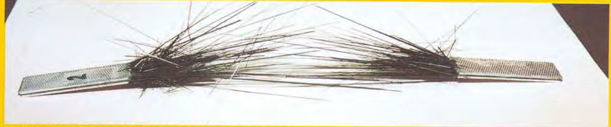
Sample after loading with failure load
